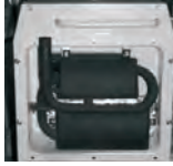
2. Remove Dual Muffer System
